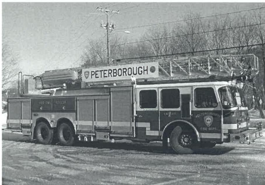
Peterborough's newest apparatus: 100-ft. E-One Aerial Ladder Truck, equipped with state-of-the-art firefighting and rescue equipment, 2005.
